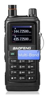
**Frequency Scan & Copy:** Enable this radio's scan function, and place it near the radio you want to scan, upon radio transmission, UV-17R Plus will display the frequency(±2.5 PPM), CTCSS or DCS tones, or 'NONE' if CTCSS or DCS is absent.
