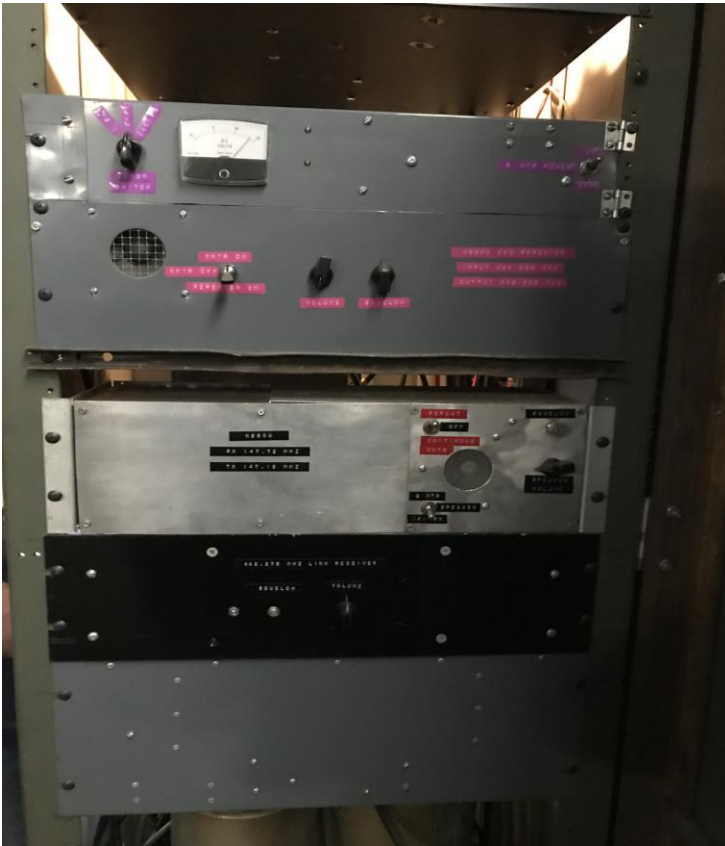
The meter panel was moved up and the repeaters removed
