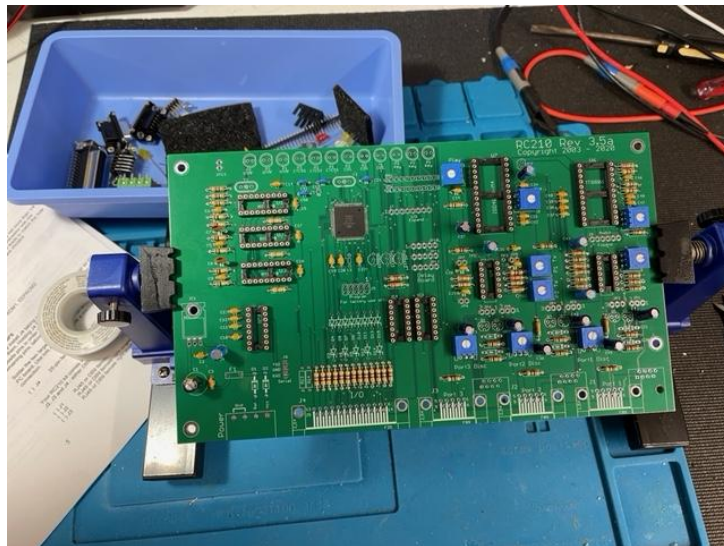
Arcom RC210 Controller build is in process
