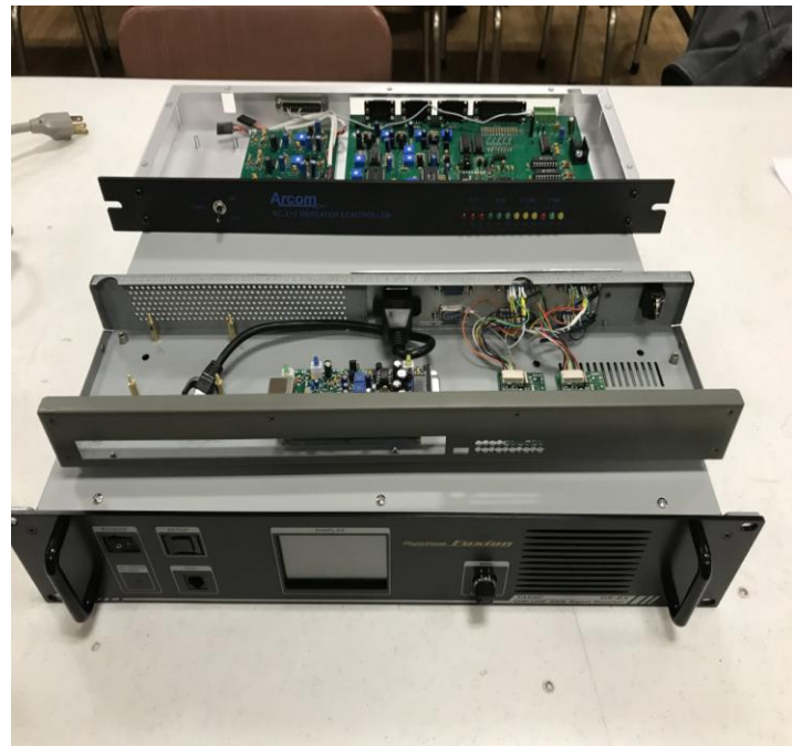
Top view of repeater Arcon controller is the chassis in the back top KC9MZ photo
